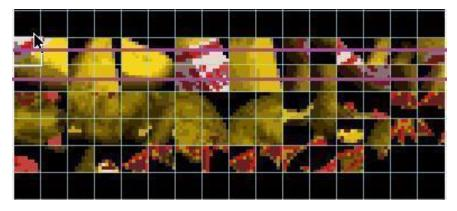
Size to send to vram shifted 5 times (dma group 1) --> In this example 2 VRAM rows are used with no 'garbage cells'. Meaning the rows are filled with no space between tile groups and no left over garbage cells. This also means there is only 1 DMA group. The size of DMA group 1 is 0x20 (which is the size of all char groups). A sprite will always have at least 1 DMA Group. There is never a DMA Group 3.
